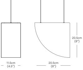
\* Components drawn in relative scale. Refer to CAD files for accurate drawings.
