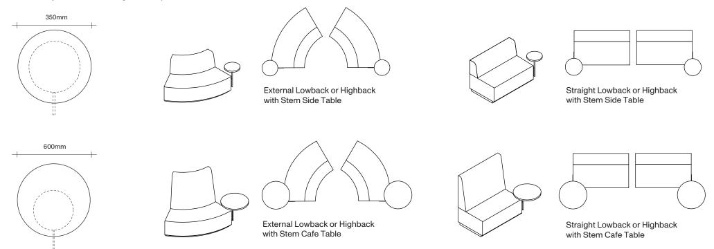
The Stem Table can be fixed to either side of any unit in the Boundary system.
