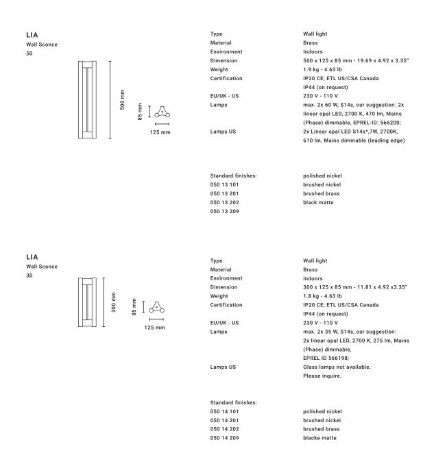
On very rare occasions, these lamps may appear to have a slight buzzing or flickering. As is the case with all retro LED lamps, this is likey casued by a number of outside influences such as incorrect installation, wiring, dimming or transformers and in some instances low electrical resistance.
