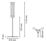
Туре Floor light Material Brass Environment Indoors Dimensions 370 x 1170 mm Cable Length 1500 mm Weight 2.4 kg Certification IP20 CE EU/UK 230 V
