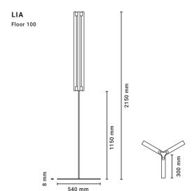
Туре Floor light Material Brass Environment Indoors Dimensions 540 x 2150 mm 1500 mm Cable Length Weight 3 kg Certification IP20 CE EU/UK 230 V
