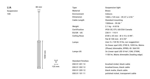
On very rare occasions, these lamps may appear to have a slight buzzing or flickering. As is the case with all retro LED lamps, this is likey casued by a number of outside influences such as incorrect installation, wiring, dimming or transformers and in some instances low electrical resistance.
